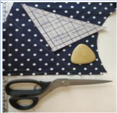
Use tailors chalk to mark around your templates onto the fabric. Cut them out using fabric scissors.
