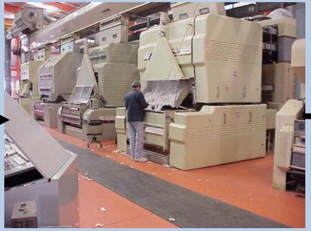
This machine – a Cotton Gin - separates the seeds from the cotton fibres.
